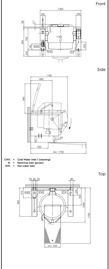
ProThermetic Sprint Electric Tilting Boiling Pan, 150lt Hygienic Profile, Freestanding
